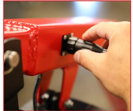
Connect receiver cord with quick connector on the side of boom arm (B) and turn on battery. Turn on remote using switch on the back. Use the remote to adjust boom arm to a level position.
