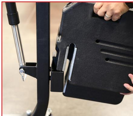
Carefully add counterweights (M), by lifting each counterweight and placing into bracket on the backside of the base arm (C).
