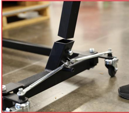
Take the base arm (C) with bracket facing out and place it into the opening on the base and legs (J). Tighten bolt to secure.
