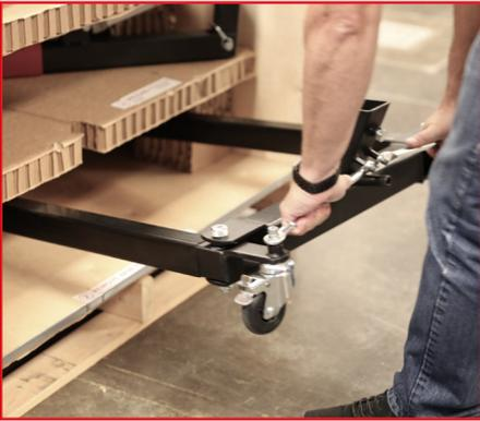
Remove parts from shipping crate in the order directed. Lock wheels on base (J) to provide stability.
