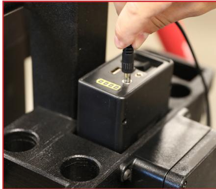
Slide battery (I) into power box (D). Plug in receiver to the battery in the 24V In/Out outlet.
