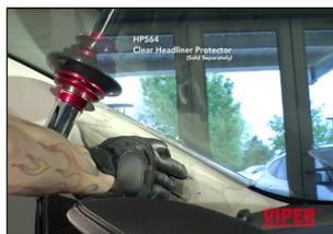
About halfway up the A-pillar you will need to reposition the Viper™ in order to complete the cut up the A-pillar and to start across the top.
