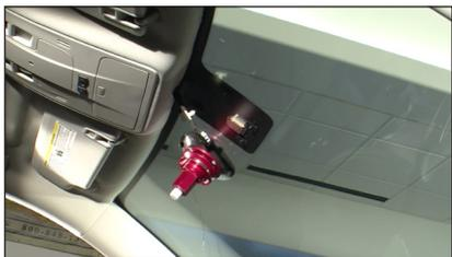
Once you reach the top corner, you most likely will encounter the clip/setting pin that was mentioned earlier on. At this point, you will use one of the two methods listed to cut the clip/setting pin.
