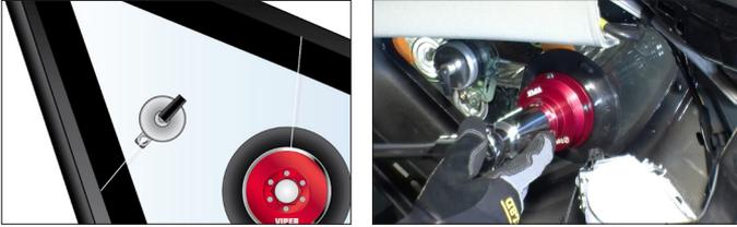
As you begin cutting again, keep in mind that the glass is now loose, so slow and easy movements are required. If not, you could pop the glass out too soon causing damage to the glass and/or body of the vehicle. Be sure to keep an 80° or less angle at all times from the Viper™ thru the urethane to the mini anchor cup. The lower degree of angle increased cutting action and makes cutting easier.
