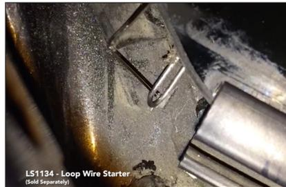
Note: To avoid damages to the painted area it is recommended to place a piece of tape on the exterior of the pinchweld.
