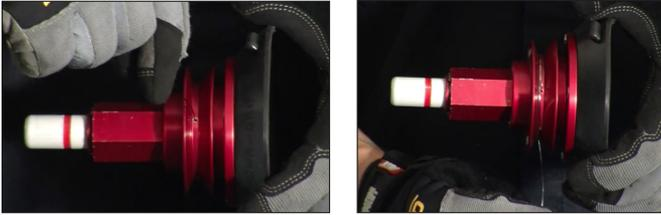
Install the Viper™ on the quarter glass at the furthest spot from the wire insertion point.
