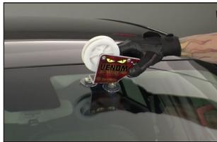
Continue to insert the wire from the Venom™ under the moulding all the way around the windshield until you are where the wire was inserted through the urethane.
