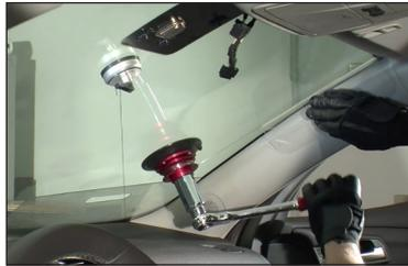
A little ways down the A-pillar you will need to reposition the Viper™ in order to continue the cut at the proper angle.
