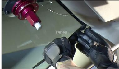
Once the clip/setting pin is cut, you can then continue cutting across the top of the windshield.
