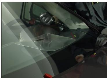
Attach the wire to the mini anchor making sure that the tab is pointed towards the original entry point of the wire.
